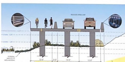
D8: ELEVATED ROAD ON CAUSEWAY (D-D')
