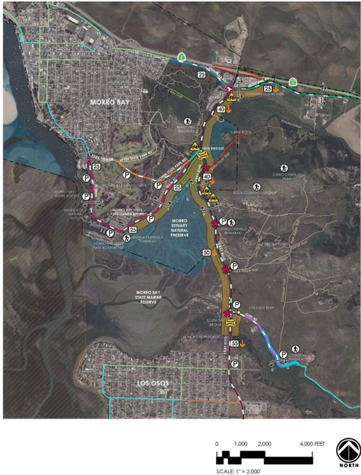
Figure 13. Plan View of Adaptation Options, including Cross Section Locations. Legend is presented in Figure 14 (below).
