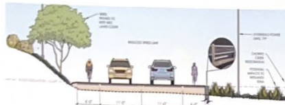
B2: ELEVATED ROAD AND CLASS I BIKE PATH ON BERM (B-B)
