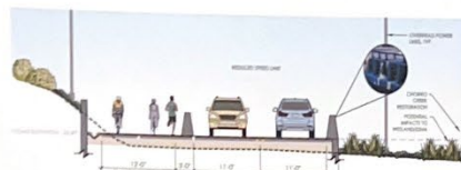
B1: ELEVATED ROAD AND CLASS II BIKE LANES ON BERM (B-B)
